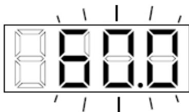
If it is necessary to change this parameter, press and hold one of the "+" (increase) or "-" (decrease) buttons to the desired value while the display flashes (5 seconds). To store the newly selected limit, wait (5 seconds) until the microcontroller exits the
