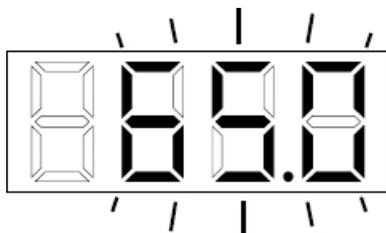
If it is necessary to change this parameter, press and hold one of the "+" (increase) or "-" (decrease) buttons to the desired value while the display flashes (5 seconds). To store the newly selected limit, wait (5 seconds) for the microcontroller to exit edit mode, which will be confirmed by the display stopping flashing and going to the current temperature value.
