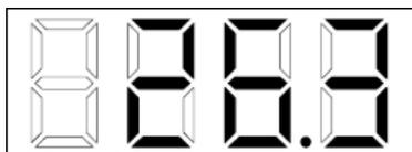
Displaying and setting the upper limit (cut-off threshold). To display a pre-set upper temperature limit (the value at which the heating will switch off), press the "+" (up arrow) button - the display will go into flashing mode (edit mode), showing the height of the upper limit. The example in the figure is 65°C.
